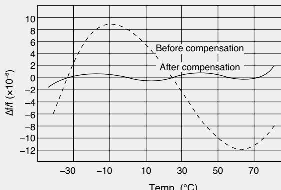
Figure 1 Example of the frequency-temperature characteristic of a temperature-compensated crystal oscillator
