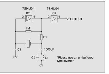
6. Frequency Range : 16 to 80 MHz max Overtone Order : 3rd, 5th overtone Load Capacitance CL : Series resonance
