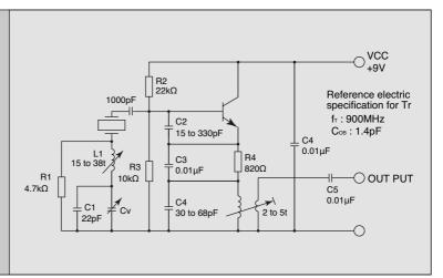
7. Frequency Range: 80 to 140 MHz max Overtone Order: 3rd, 5th overtone Load Capacitance CL: Series resonance
