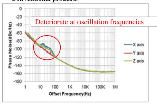
Test conditions: IEC 60068-2-64 5 to 100 Hz random oscillation  $2.0 \times 1.6$ mm 26 MHz
