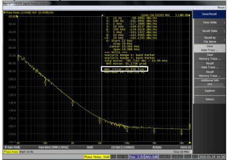
Condition: Nominal frequency 156.25MHz, LVDS output, power supply voltage [ $V_{CC}$ ] +3.3V,
