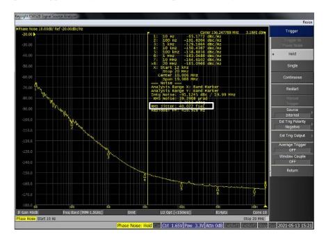
Conditions: Nominal frequency 156.25MHz, LVDS out, power supply voltage [VCC] +3.3V, temperature +25deg.C
