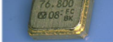
76.8 MHz crystal units with built-in thermistor
