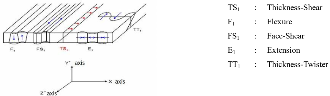
Fig. 1 Vibration mode of AT-CUT crystal unit
