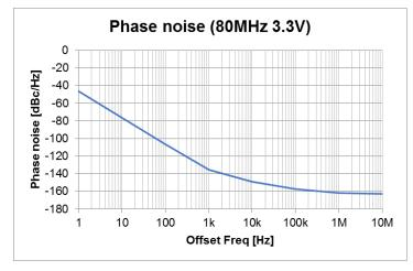
• Phase jitter : Typ. 100 fs (Frequency Offset: 12 kHz to 20 MHz) @80 MHz, 3.3 V
