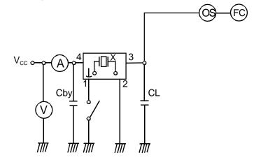
CL ; 15pF MAX including input capacity of oscilloscope Cby ; Bypass capacitor (0.01uF)
