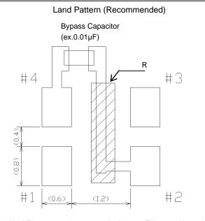
Note) Please mount bypass capacitor(ex.0.01 $\mu$ F) between Vcc and GND (close to the product) to keep stable operation. Please reserve a large ground pattern on the PCB where the oscillator is installed.
