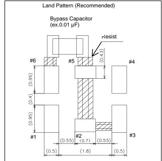
Note) Please mount bypass capacitor(ex.0.01µF) between Vcc and GND (close to the product) to keep stable operation. Please reserve a large ground pattern on the PCB where the oscillator is installed.
