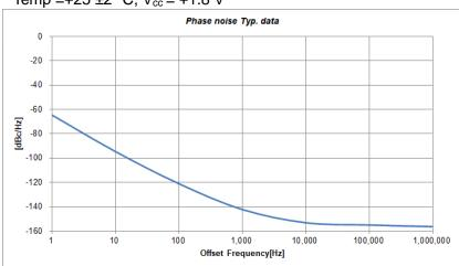
Temp =+25  $\pm$ 2 °C,  $V_{cc}$  = +3.3 V
