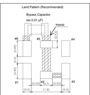
Note) Please mount bypass capacitor(ex.0.01µF) between Vcc and GND (close to the product) to keep stable operation. Please reserve a large ground pattern on the PCB where the oscillator is installed.
